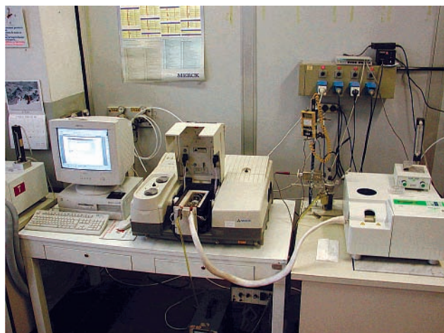
Figure 10. Picture of the equipment (TG + FTIR) used to identify the decomposition products.
